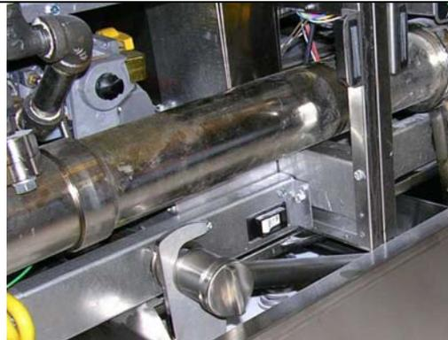
Recirculation system is to be added to fryer containing filter pump.
