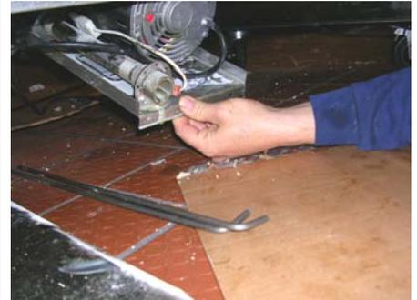
Lower pump assembly out of cabinet, motor end first.
