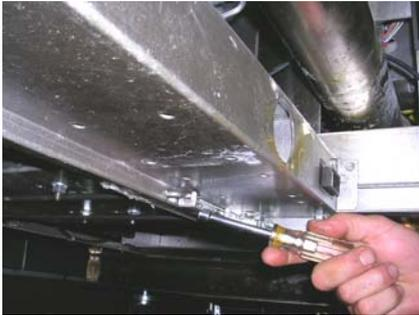
Remove filter pan socket, and retaining bracket from pump support rods.
