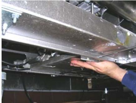
Support pump assembly with hand as shown while removing pump support rods with other hand.
