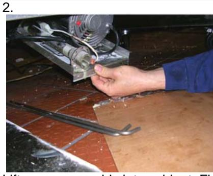
Lift pump assembly into cabinet. Flex hose goes on top of gas line.
