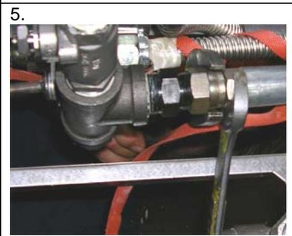
Attach hose, tighten with 2 wrenches to prevent twisting pump hose.
