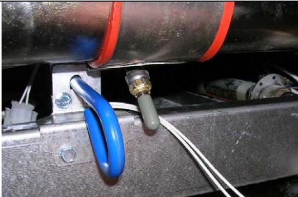
**Shortening Recirculation System Operator Handle**-Pulling blue handle starts pump and shortening is recirculated in the filter pan.
