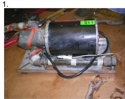
Wrap pump electrical leads as shown to prevent pinching.
