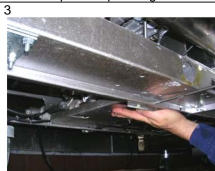
Slide support rods through holes in cabinet cross member and pump mounting plate.
