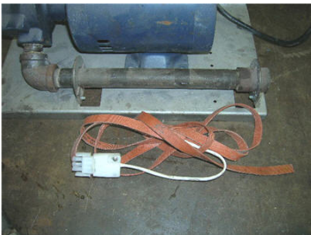
Step 11. If fryer is equipped with heat tape, cut existing white heat resistant tape in order to remove heat tape from pump assembly. Discard heat tape.
