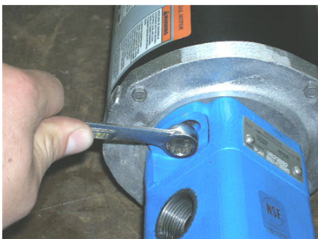
Step 23 Loosen pump head mounting bolts (qty-2) with the 1/2" wrench (do not remove)
