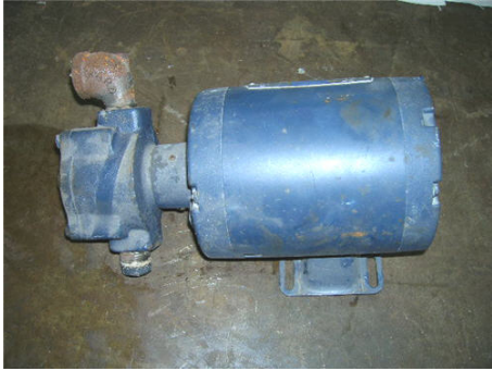
Haight pump shown with fittings that will not be needed.
