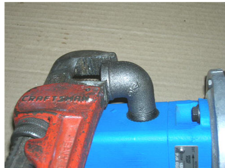
Step 16B (Viking Pump Replacement Only) Remove 3/4" npt street elbow from Viking pump outlet port using large adjustable pipe wrench.
