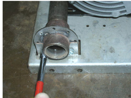
Step 24. Set pump on pump plate, rotate both pump head and inlet supply nipple until mounting holes align. Screw coupling to plate using qty-2 10-24 self tapping screws with variable speed drill with 5/16 hex bit.
