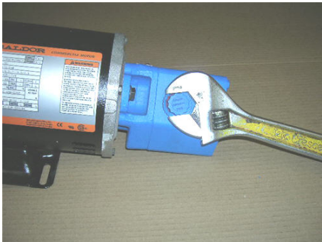
Step 21. Locate parts from replacement kit. Remove the plastic thread/gear protective caps from pump (kit item 1) with the large adjustable wrench.
