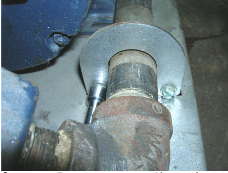
Step 13. Remove two self tapping screws attaching the U-bracket to pump plate assembly using the variable speed, reversible drill with 5/16" hex bit.
