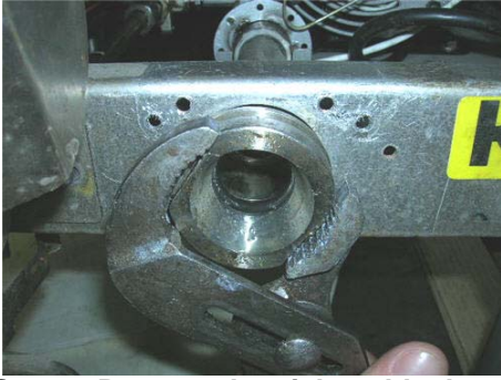
Step 7. Remove the pick up block weldment using the large slip joint pliers. Can also be removed by clamping on 3/4" npt nipple.
