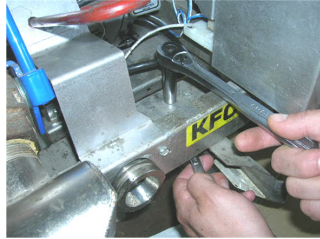
Step 48. Reassemble right filter rail with qty-4 1/4-20 bolts, washers and nuts using the 7/16" open end wrench and 7/16" socket and ratchet.
