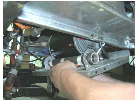
Step 10. Slide pump assembly to the left and lower left hand side of pump assembly. Use caution that no wires or power supply cables are pinched. Remove pump assembly from cabinet.
