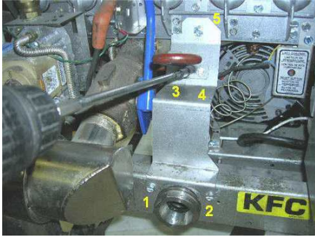
Step 47. Assemble polishing brackets to polishing handle and fryer using qty-5 10-24 self tapping screws with the variable speed reversible drill with 5/16" hex bit.
